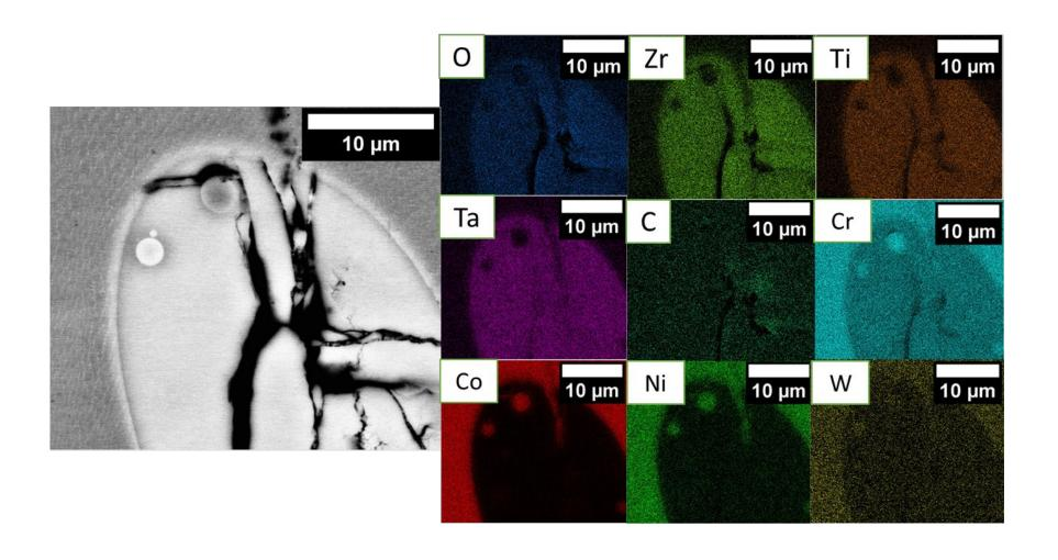
EDS analysis reported excess oxygen, aluminum, titanium, zirconium, and tantalum within the agglomerate particle, pointing towards diffusion of these elements into the oxide followed by oxidation of elements in the matrix. These supports the conclusion that the particles seen in EDS are oxide agglomerates
