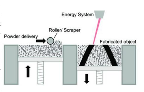
temperatures, and are often used in high stress, high temperature applications such as gas turbine blades. Compared to traditional casting methods, LPBF can produce parts with high levels of detail, with retained strength and ductility due rapid solidification rates.
